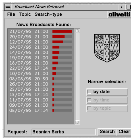
Statistical Information Retrieval methods are used to rank potentially relevant news broadcasts for a given request.
