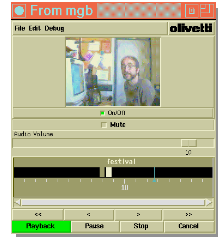
In the browser the horizontal timeline shows potential word hits, highlighting each word. Random access playback can be initiated by clicking anywhere in the timeline.
