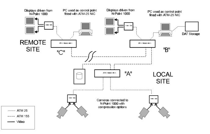
Recorded information is buffered in the hard disc, and can be downloaded to DAT tape on a timed interval basis. Information can be retrieved from the hard disc and displayed directly on one of the monitoring points. Also it will be possible to identify which DAT tape contains information from the last 28 days, as the hard disc will contain a catalogue of what was recorded.
